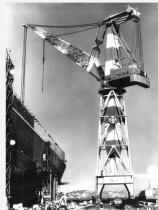
1971: 125 t rotary crane by Krupp for the shipyard of Mitsui Shipbuilding in Tamano.
